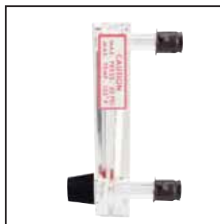
Model MMF mounts easily from front of panel. Drill two 1/32" or 1/16" dia. holes in panel on 2 1/16" centers. Insert mounting connector spuds. From rear, slide on the two spring retainers (furnished) and push on rubber or plastic tubing.
